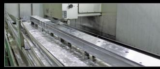
Mirror surface grinding of long workpiece
