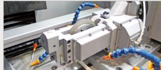
Workpiece indexing unit (option)
