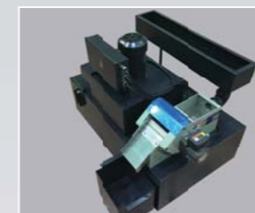
Coolant and Dust Suction System with Magnetic Dust Separator
